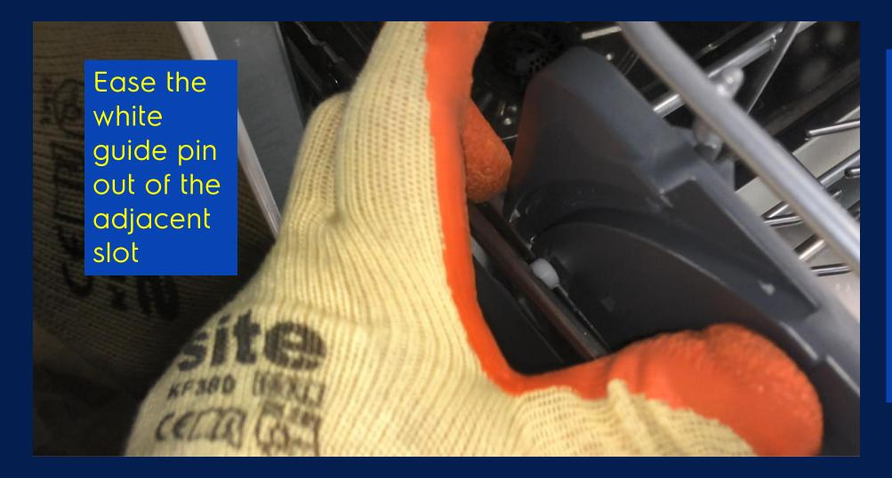
Apply opposing pressure onto the basket and side rail until the white pin is clear
