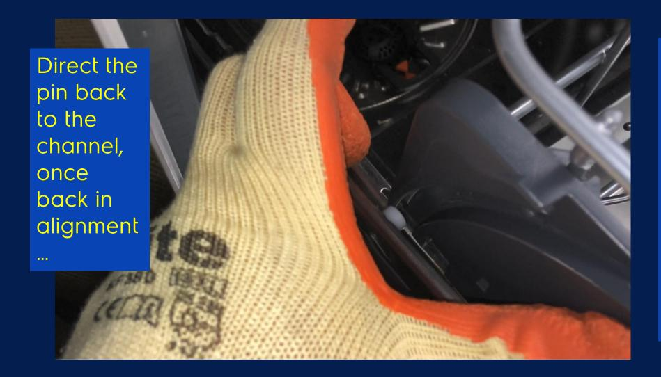
...release the applied pressure to drop the white guide pin back into the correct position.
